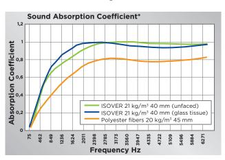
\*Sound Absorption Coefficient according to ISO 10534-2
