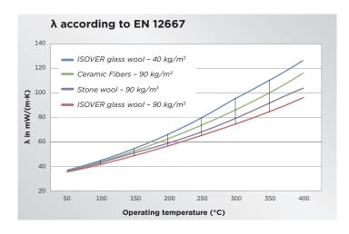
ISOVER is your partner to develop high-performing solutions to reach the highest energy efficiency classes. Our R&D teams provide testing facilities as well as tailor-made supports for you to develop tomorrow's cooking solutions.
